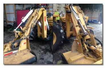
Other projects include a hydraulic jack hammer for the backhoe. A priceless tool in the winter or concrete roadway situations. A large capacity water truck (Mack, naturally) >>>
