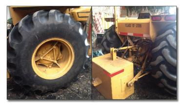
An old rotary mower was beefed up to be used but how to join the tractor and mower? With the exception of the hydraulic cylinders, Mike designed and fabricated each piece of material between the mower deck and the tractor. Some angle adjustment was made to lock the deck in a raised-stowed position. The attention to detail matches any commercially manufactured units I have seen.
